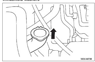
The windshield washer reservoir is in the engine compartment. Check the fluid level at regular intervals and replenish the fluid if necessary.
